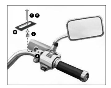
STEP 2: Install the Heat Controller Bracket <sup>B</sup> using screw <sup>O</sup> or <sup>D</sup> and spacers <sup>D</sup> as shown above.
