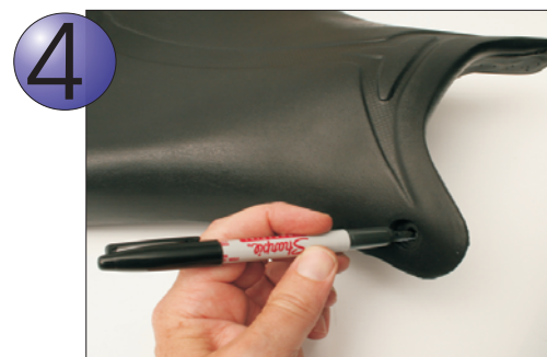
PLACE THE SPEED SEAT ON TOP OF THE PAN, MAKING SURE IT IS CORRECTLY ALIGNED AND FITTED TOGETHER. HOLD THE AREA TO BE MARKED WITHOUT SHIFTING THE PAD AROUND. MARK A CENTER SPOT IN EACH HOLE. IMPORTANT: CHECK FOR CORRECT ALIGNMENT BEFORE DRILLING.
