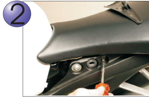
PULL OFF SIDE PANEL STARTING AT THE BACK POINT. REMOVE BOTH PHILLIPS SCREWS (ONE EACH SIDE).
