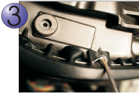
WITH A PUNCH OR FLAT HEAD, PRY UP THE STAPLES. USE PLIERS TO REMOVE THEM. REMOVE COVER AND FOAM.
