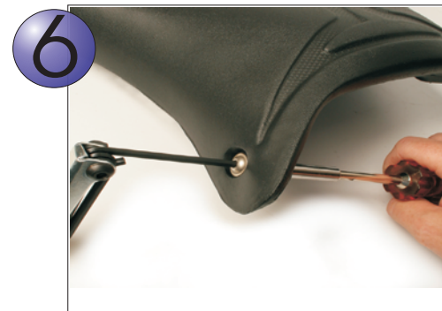
SNUG EACH NUT BUT DO NOT OVER TIGHTEN AND SMASH SEAT MATERIAL TOO MUCH. REINSTALL SEAT. NOW GO RIDE AND GET LOOKS!
