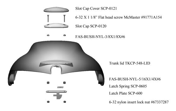
Dry fit slot cap cover SCP-0121 before gluing it onto PAINTED PODS to make sure it will slide and spring back freely after gluing. Sand slot cap SCP-0120 more if needed then glue into place.
