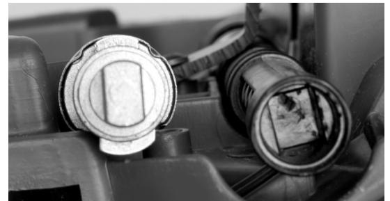
Lock barrel (left) fits into the notched latch rod (right).
