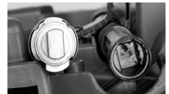
Lock barrel (left) fits into the notched latch rod (right).
